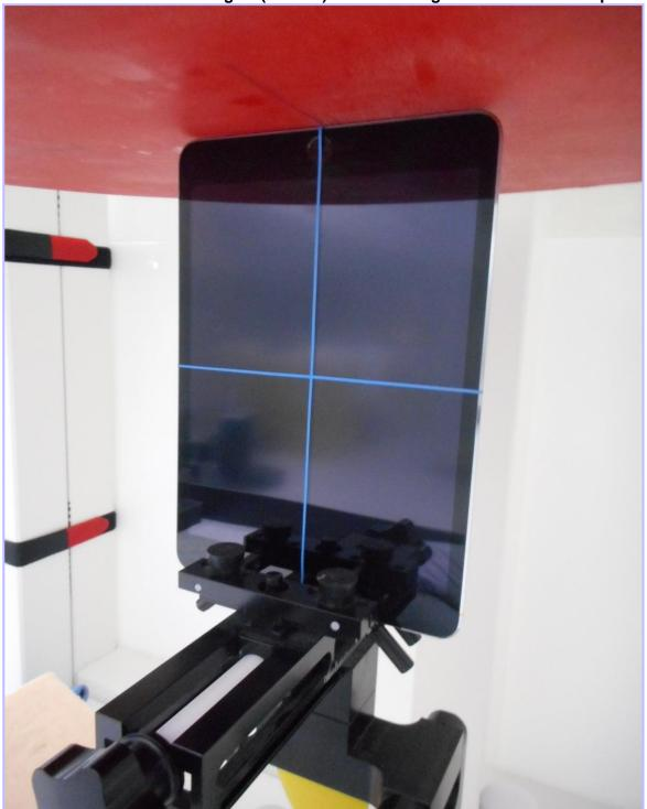
PHT/10407443JD13A/005: Edge 4 (Left Hand Side) of EUT Facing Phantom at 0mm Separation
