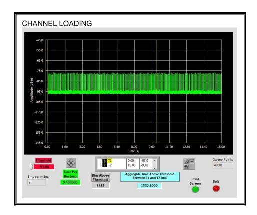
The level of traffic loading on the channel by the EUT is 15.52%
