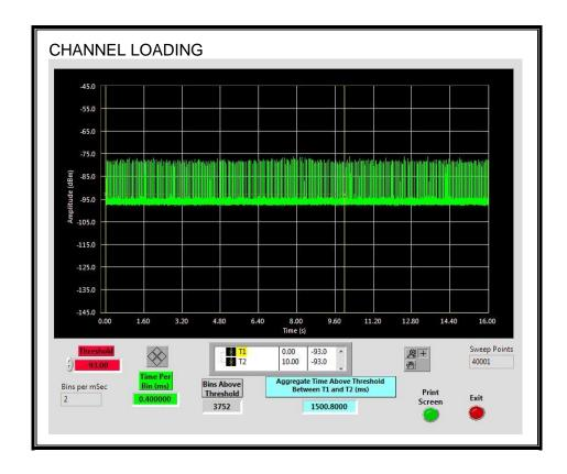
The level of traffic loading on the channel by the EUT is 15.0%
