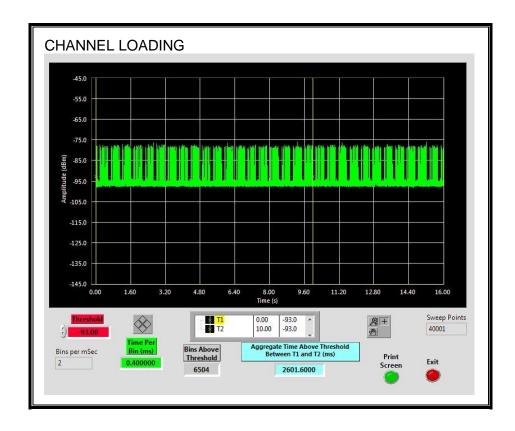
The level of traffic loading on the channel by the EUT is 26.016%
