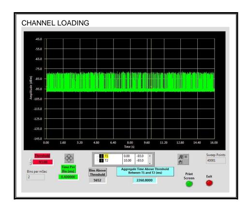
The level of traffic loading on the channel by the EUT is 22.608%
