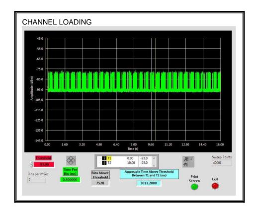
The level of traffic loading on the channel by the EUT is 30.11%
