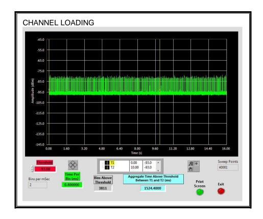
The level of traffic loading on the channel by the EUT is 15.24%
