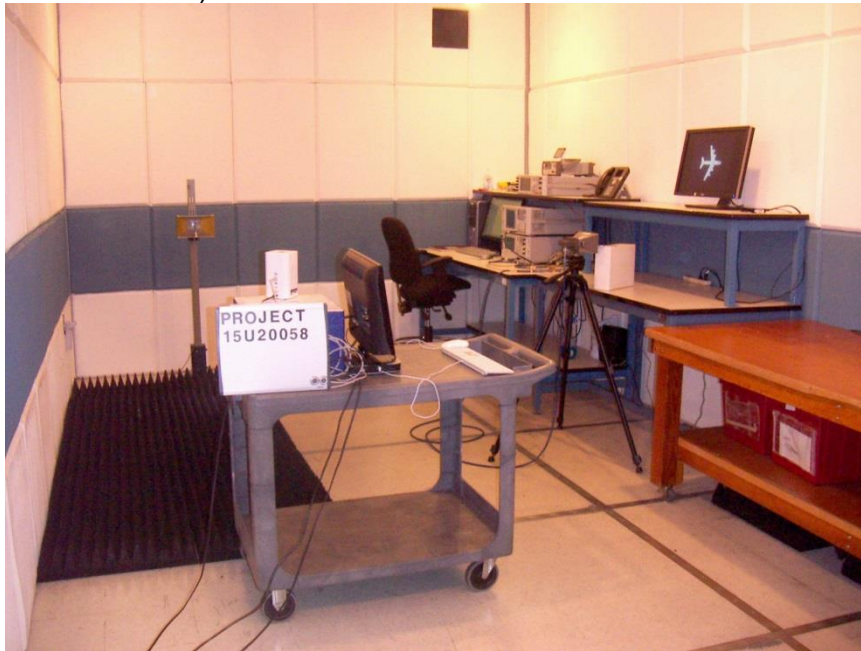
DFS FRONT PHOTO (CLIENT-TO-CLIENT COMMUNICATIONS MODE SETUP)
