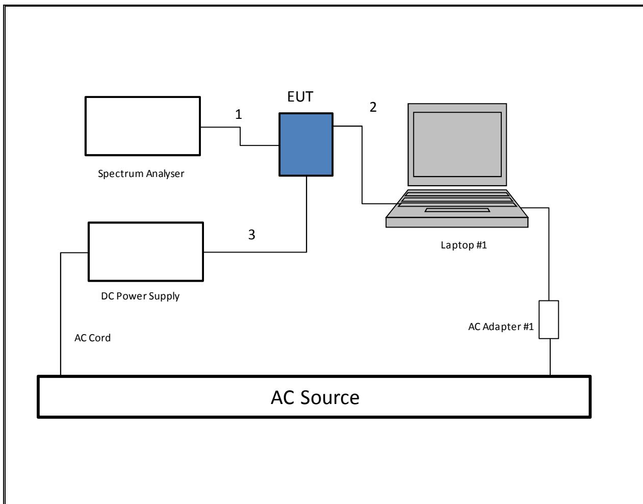
**TEST SETUP- RADIATED-ABOVE 1 GHZ**
