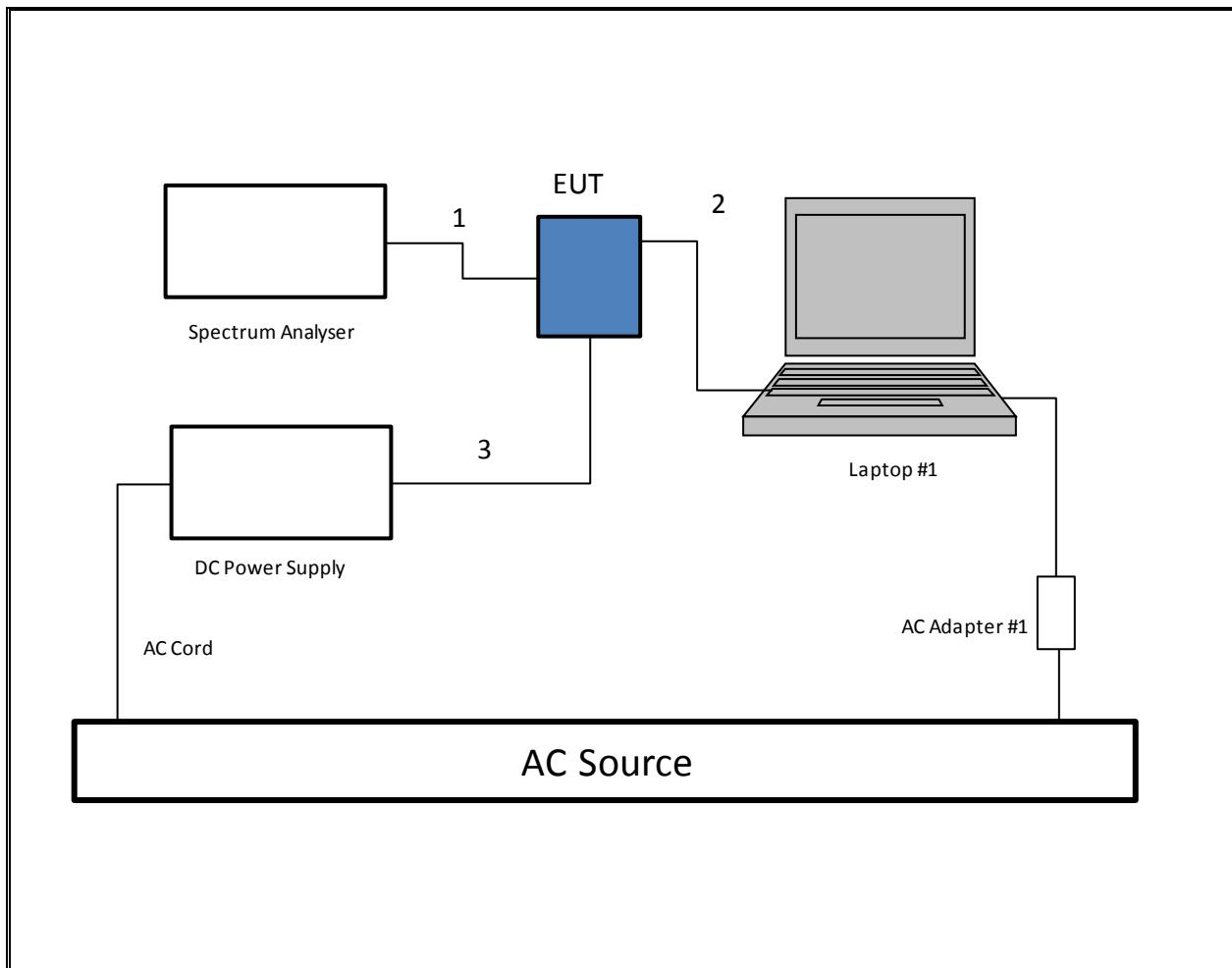
**TEST SETUP- RADIATED-ABOVE 1 GHZ**
