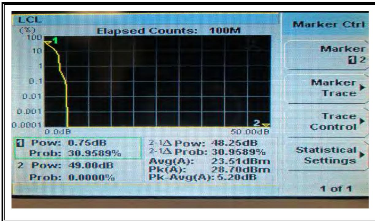
16QAM Band 4 (1.4 MHz BAND WIDTH)
