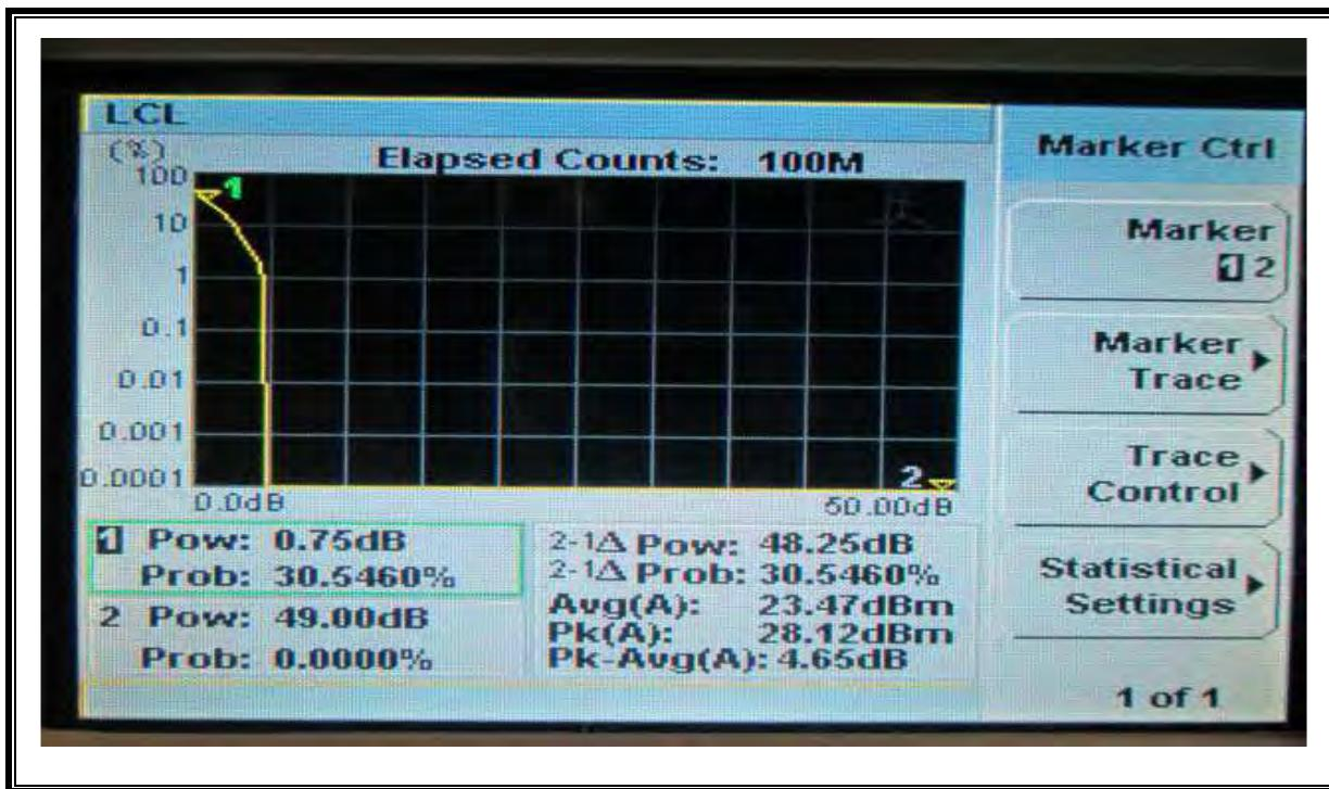
LTE 16QAM Band 4 (20 MHz BAND WIDTH)
