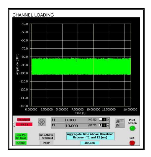
The level of traffic loading on the channel by the EUT is 40.24%
