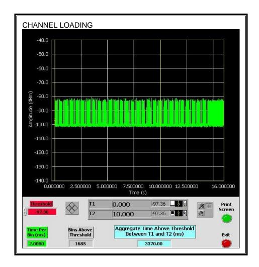
The level of traffic loading on the channel by the EUT is 33.7%
