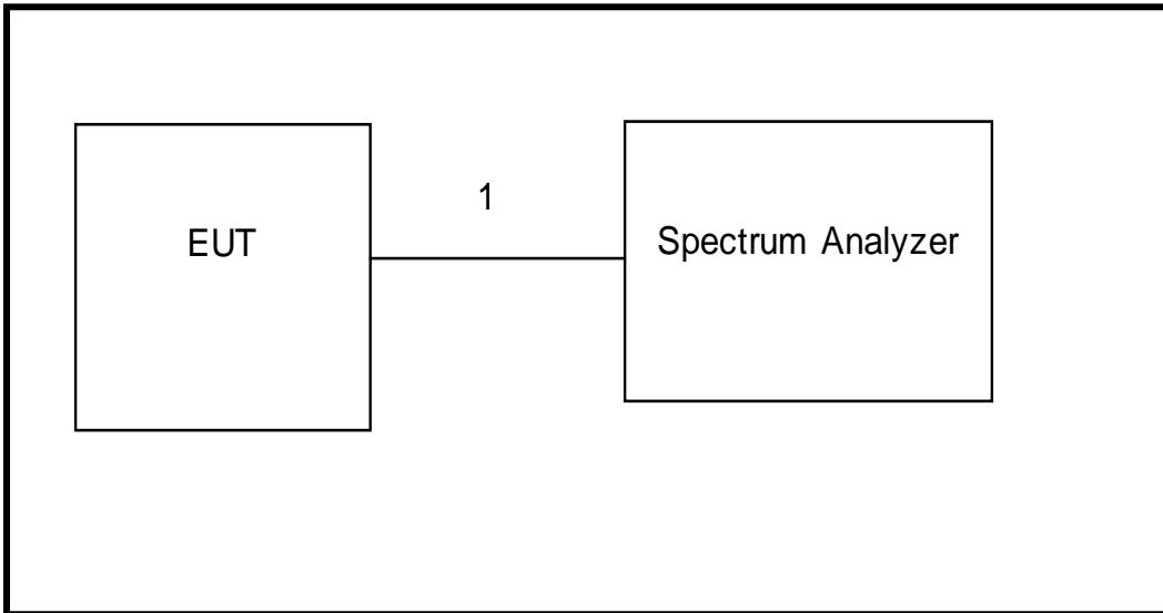
**SETUP DIAGRAM FOR RADIATED TESTS**
