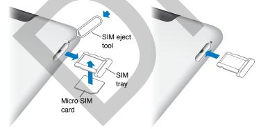
Open the SIM tray. Insert the SIM eject tool into the hole on the SIM tray, then press firmly and push the tool straight in until the tray pops out. Pull out the SIM tray to install or replace the SIM card. If you don't have a SIM eject tool, try the end of a small paper clip.
