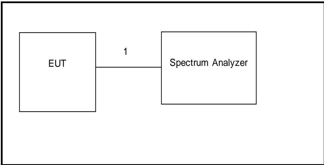
**SETUP DIAGRAM FOR RADIATED TESTS**
