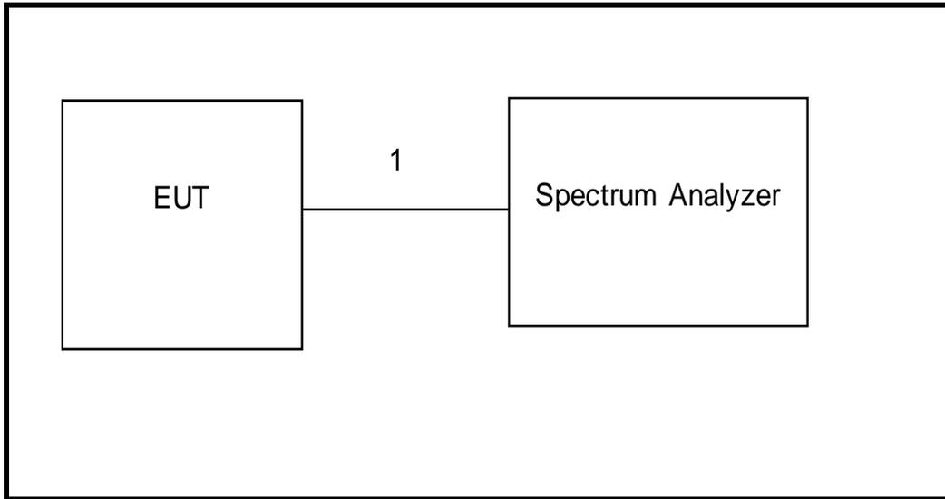
**SETUP DIAGRAM FOR RADIATED TESTS**
