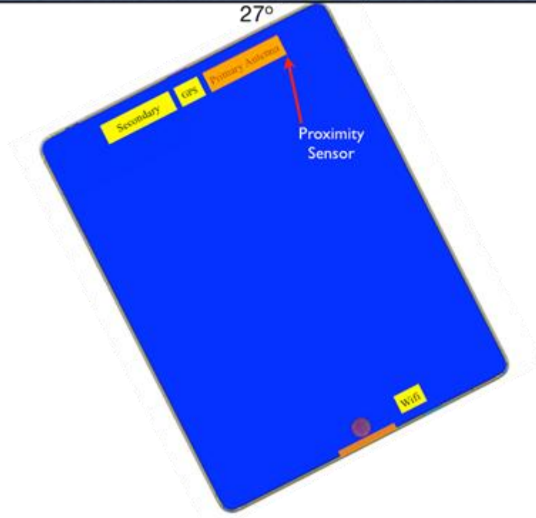
DUT angle at which second-stage is activated
