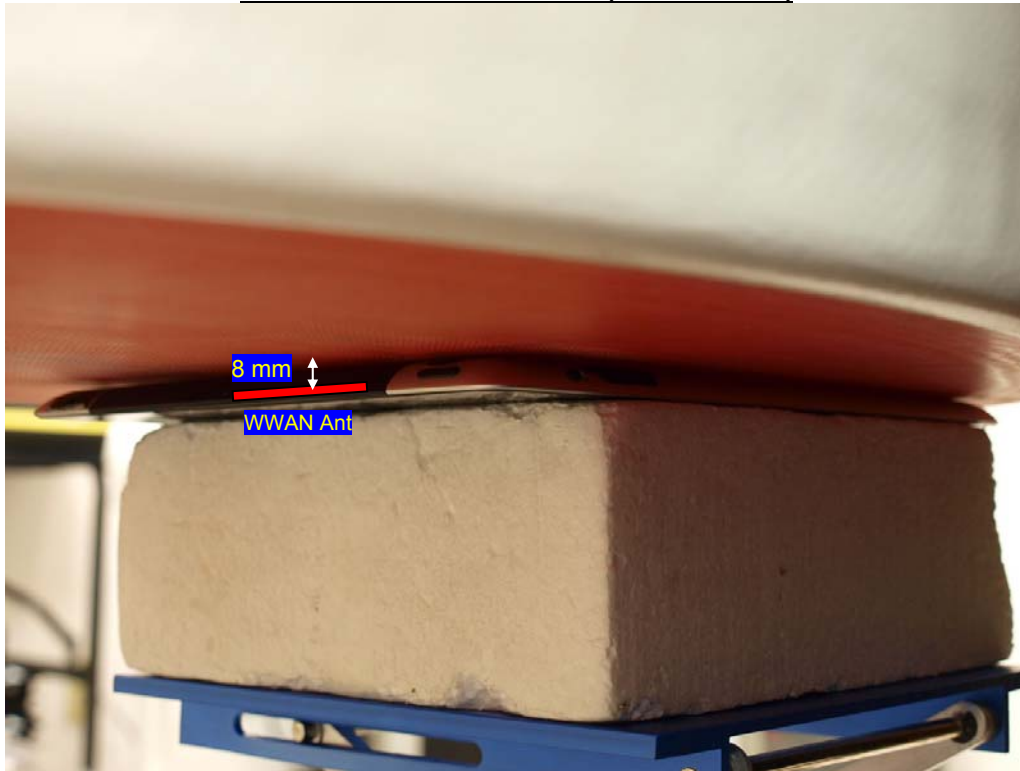
Back Surface (for PCS band) 10 mm air gap distance
