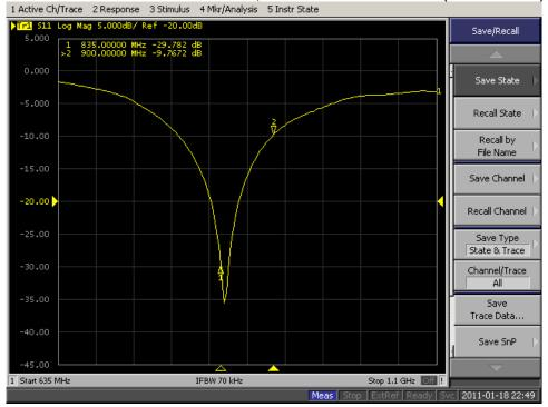
835 Body Calibrated impedance: 48.2  $\Omega$ ; Measured impedance: 48.881  $\Omega$  (within 5 $\Omega$ )
