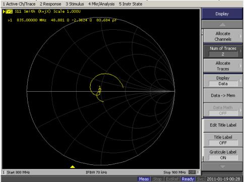
Calibrated return Loss: -28.5 dB; Measured:-29.782 dB (within 20%)
