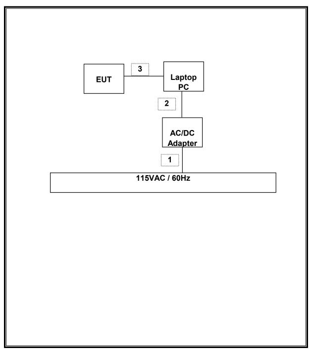
Note: Laptop PC was used to control the operation of the EUT.
