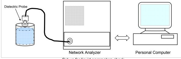
Set-up for liquid parameters check
