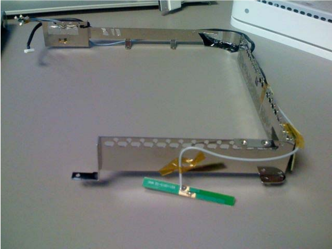
Antenna Bracket with Third Antenna
