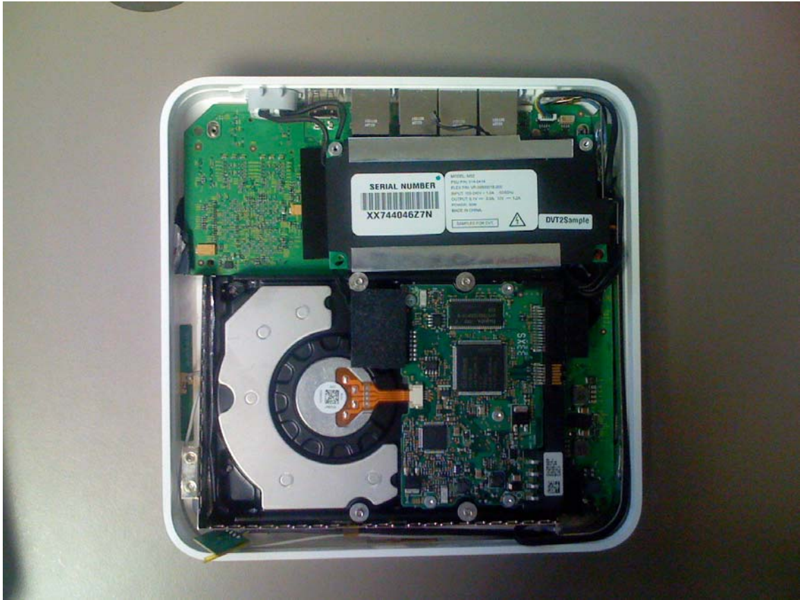
Enclosure with Shield Cover Removed
