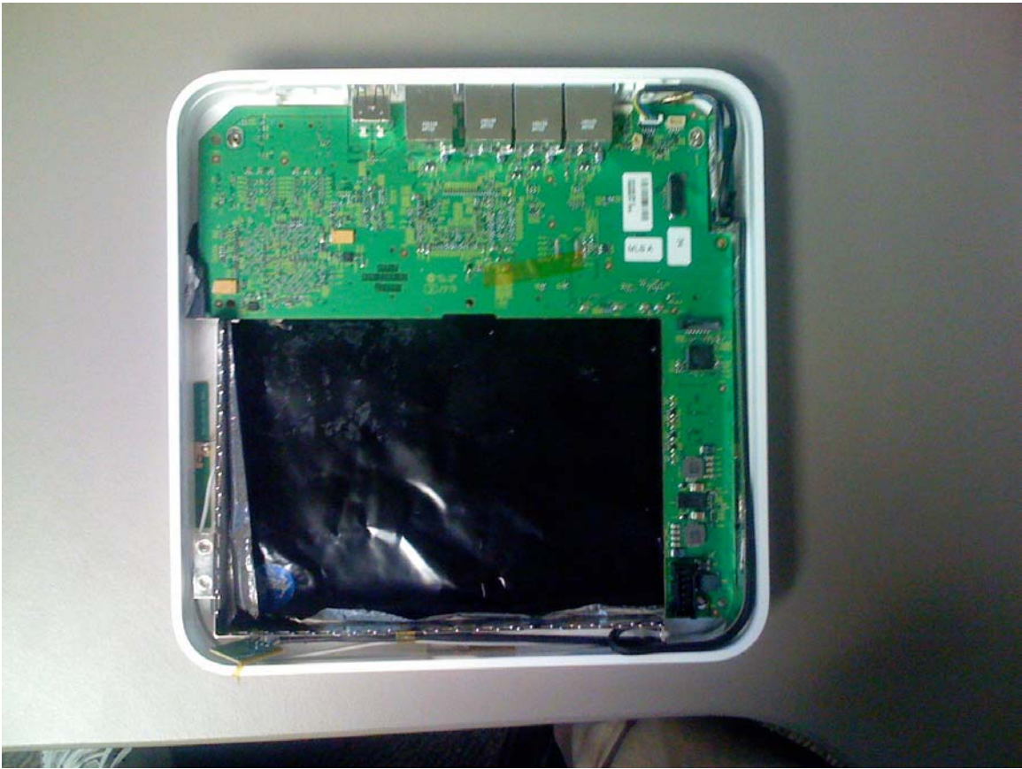
Enclosure with Hard Drive and Power Supply Removed
