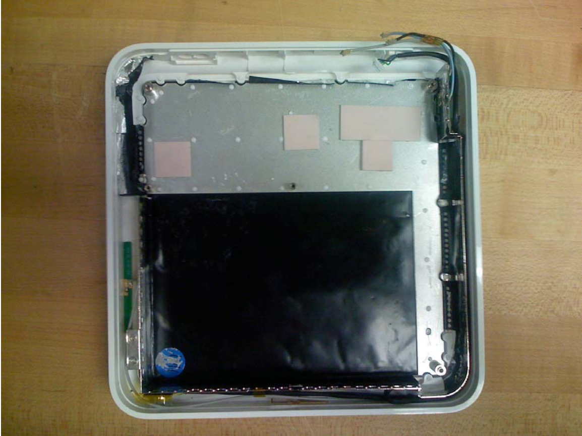
Enclosure with MLB Removed
