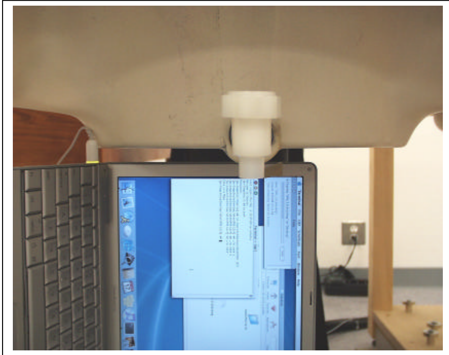
EUT Setup Configuration 1 [12" PowerBook G4 with Inverted F (603-1203) antenna] Spacing between host device and phantom - 1.5 cm
