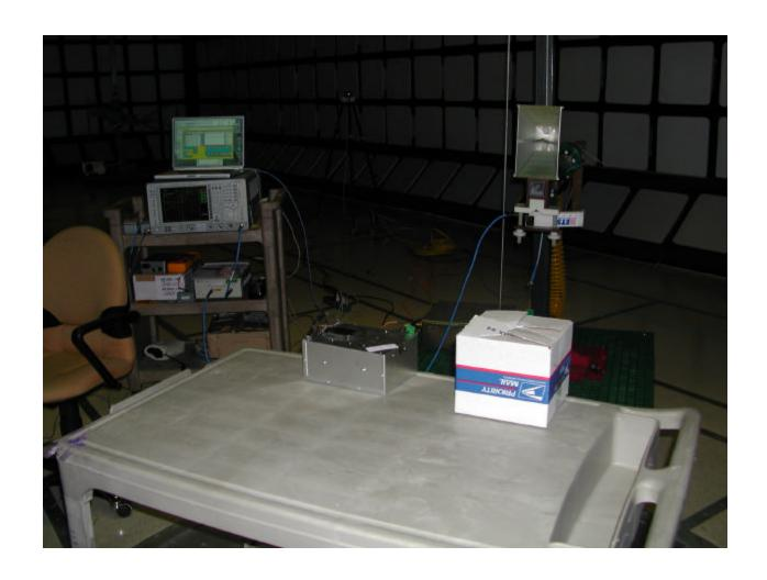
Digital Device Radiated Emission Measurement
