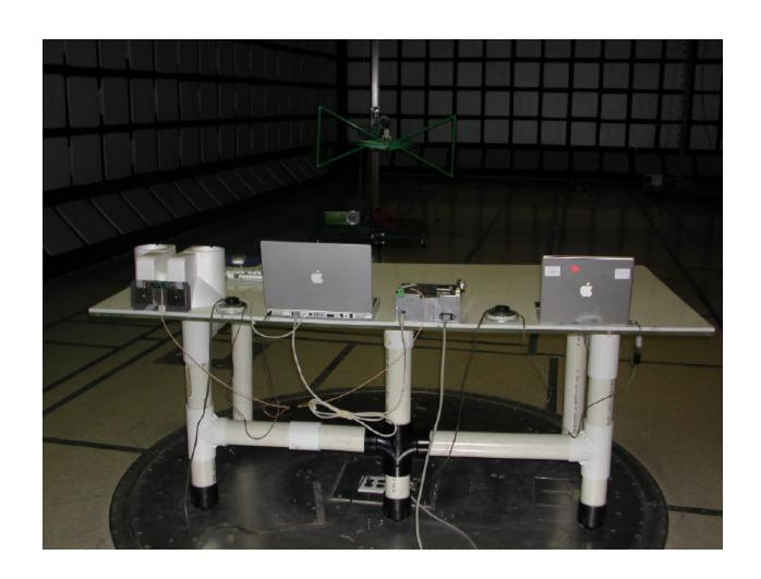
Powerline Conducted Emissions Measurement
