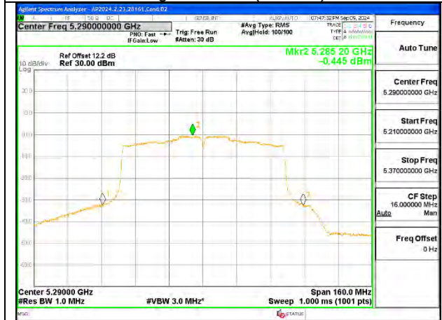
80MHz - Mid Channel (UNII-2a) – Ant 1
