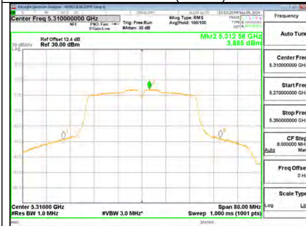
40MHz - Mid Channel (UNII-2a) – Ant 2
