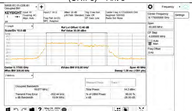
20MHz - Mid Channel – MRU106+26T-RU82 (UNII-5) – Ant 5
