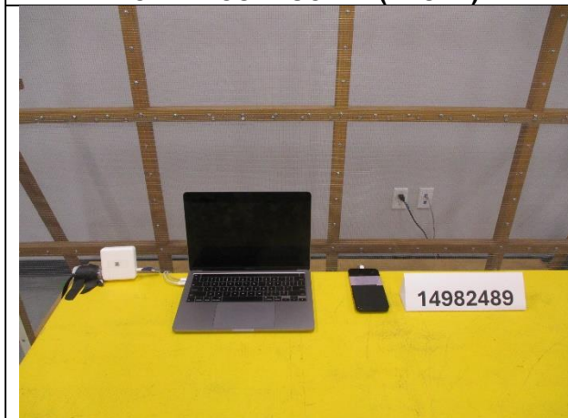
AC LINE CONDUCTED WITH HOST (FRONT)
