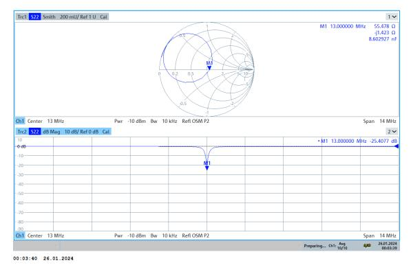
• Return/Loss is greater than the -20 dB cutoff and Impedance is within 5  $\Omega$  of previous value.
