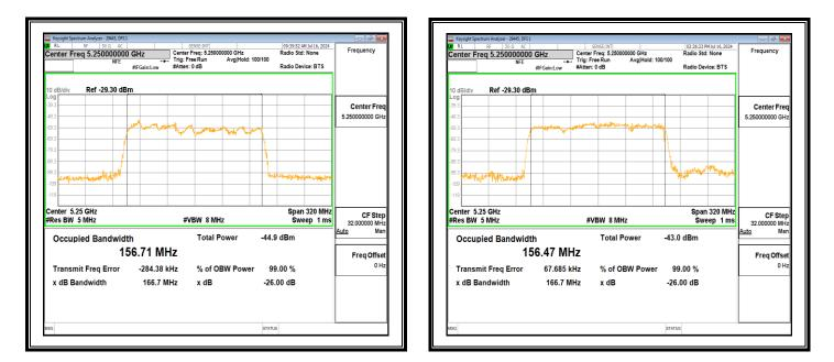
After the puncture command the same 20 MHz Sub-Channel centered at 5300 MHz is disabled by both AP and Client Device.
