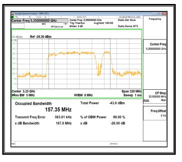
After the puncture command the same 20 MHz Sub-Channel centered at 5320 MHz is disabled by both AP and Client Device.
