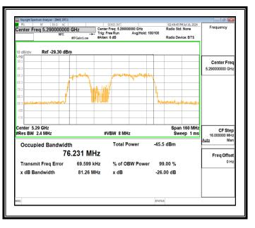
After the puncture command the same 20 MHz Sub-Channel centered at 5260 MHz is disabled by both AP and Client Device.
