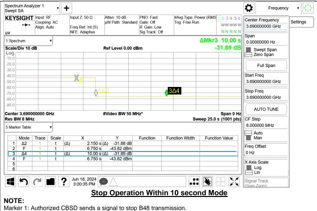
Marker 2: Time elapsed since signal to stop B48 transmission. EUD has stopped transmission.
