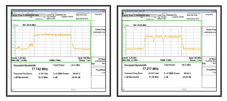
After the puncture command the same 20 MHz Sub-Channel centered at 5280 MHz is disabled by both AP and Client Device.
