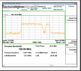
After the puncture command the same 20 MHz Sub-Channel centered at 5320 MHz is disabled by both AP and Client Device.
