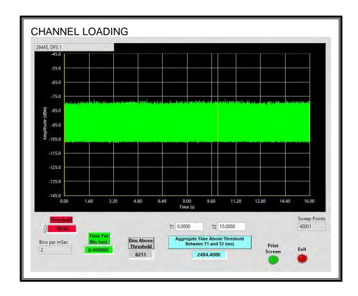
The level of traffic loading on the channel by the EUT is 24.84%
