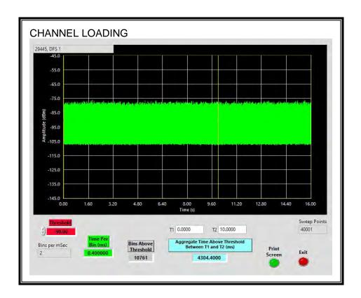
The level of traffic loading on the channel by the EUT is 43.04%
