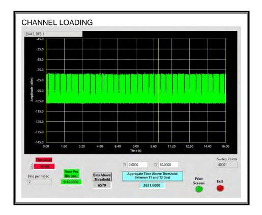
The level of traffic loading on the channel by the EUT is 26.31%
