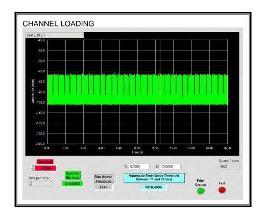
The level of traffic loading on the channel by the Peer Slave is 18.18%
