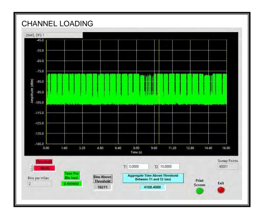
The level of traffic loading on the channel by the EUT is 41.08%
