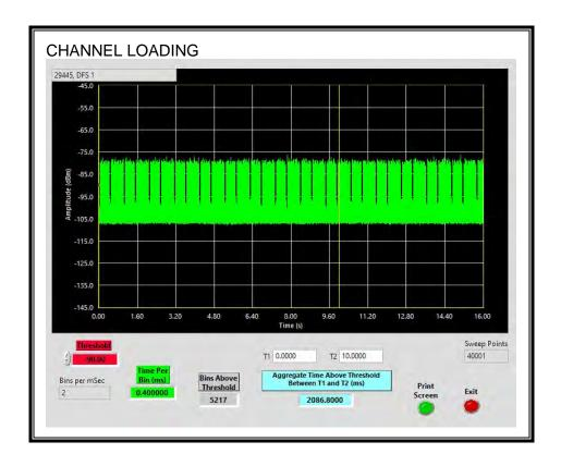
The level of traffic loading on the channel by the EUT is 20.86%
