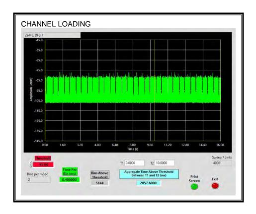
The level of traffic loading on the channel by the Peer Slave is 20.57%
