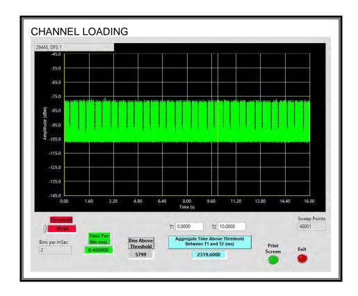
The level of traffic loading on the channel by the Peer Slave is 23.19%
