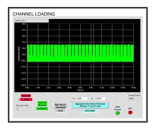
The level of traffic loading on the channel by the EUT is 24.43%
