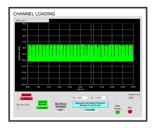
The level of traffic loading on the channel by the EUT is 21.46%
