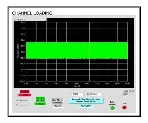
The level of traffic loading on the channel by the EUT is 49.39%
