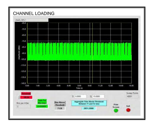
The level of traffic loading on the channel by the EUT is 28.51%
