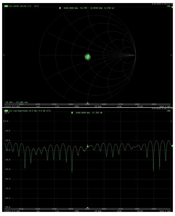
• Return/Loss is greater than the -20 dB cutoff and Impedance is within 5  $\Omega$  of previous value.
