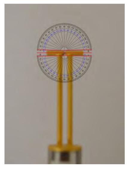
• The center red line indicates that the arms of the dipole fall within  $\pm 2^{\circ}$
