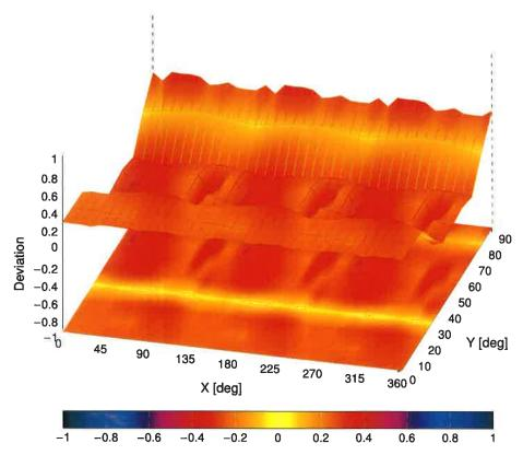
Probe isotropy for  $E_{tot}$ : probe rotated  $\phi=0^\circ$  to 360°, tilted from field propagation direction  $\vec{k}$  Parallel to the field propagation ( $\psi=0^\circ-90^\circ$ ) at 30 GHz: deviation within  $\pm 0.42$  dB Parallel to the field propagation ( $\psi=0^\circ-90^\circ$ ) at 60 GHz: deviation within  $\pm 0.39$  dB
