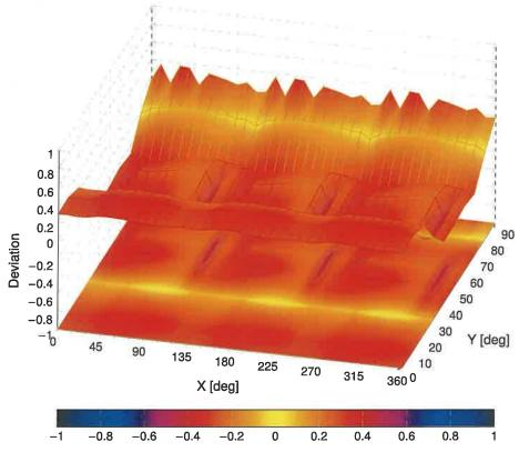
Probe isotropy for  $E_{tot}$ : probe rotated  $\phi = 0^{\circ}$  to 360°, tilted from field propagation direction  $\vec{k}$ Parallel to the field propagation ( $\psi$  = 0° - 90°) at 30 GHz: deviation within ±0.37 dB Parallel to the field propagation ( $\psi$  = 0° - 90°) at 60 GHz: deviation within ±0.41 dB
