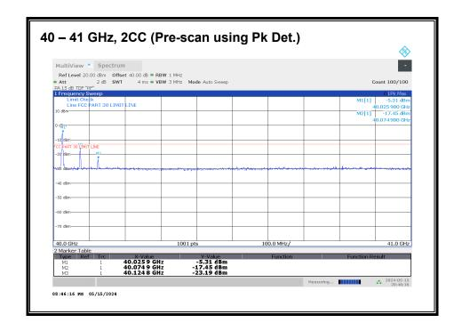
Worst case configuration: SISO-DUAL\_QPSK\_(50 MHz + 50 MHz)\_High CH\_RB Offset 1/15 (1RB-M)
