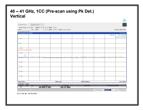
No emission detected using Peak Detection.
