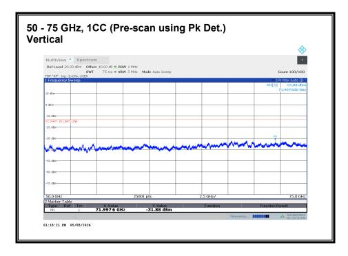
No emission detected using Peak Detection.
