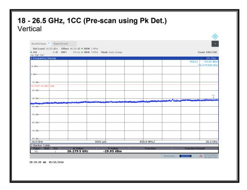
No emission detected using Peak Detection.
