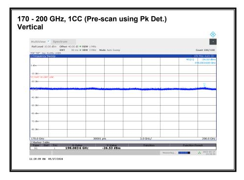
No emission detected using Peak Detection.
