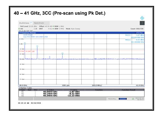
Worst case configuration: SISO-DUAL\_QPSK\_(100 MHz + 100 MHz + 100 MHz)\_High CH\_RB Offset 1/32 (1RB-M)
