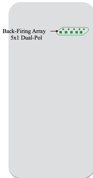
Figure 4. Schematic of the simulation model consisting of a back-firing 5G antenna array.
