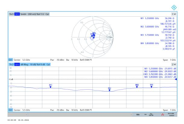
$\bullet~$  Return/Loss is greater than the -20 dB cutoff and Impedance is within 5  $\Omega$  of previous value.
