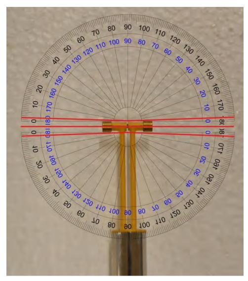
• The center red line indicates that the arms of the dipole fall within  $\pm 2^\circ$
