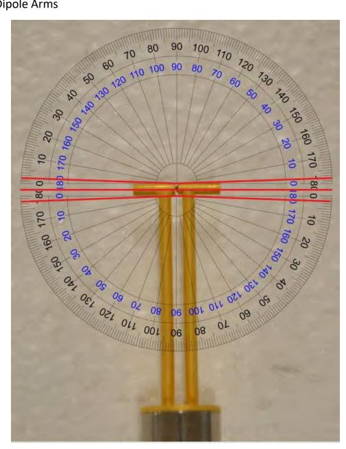
The center red line indicates that the arms of the dipole fall within  $\pm 2^{\circ}$
