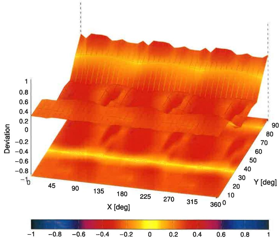
Probe isotropy for  $E_{\text{tot}}$ : probe rotated  $\phi = 0^\circ$  to  $360^\circ$ , tilted from field propagation direction  $\hat{k}$
