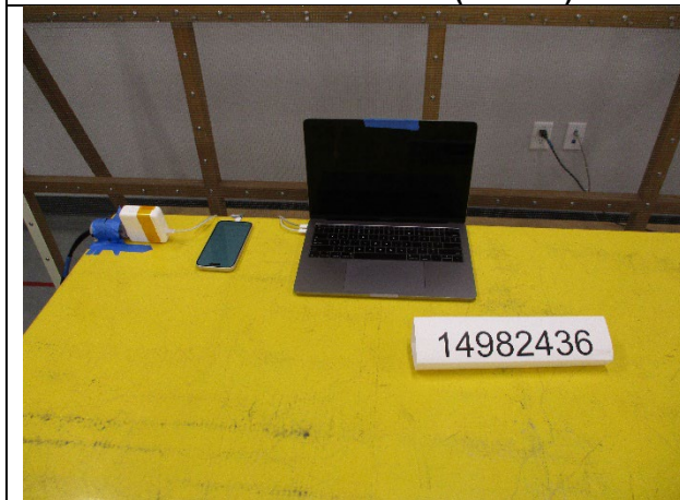
AC LINE CONDUCTED WITH HOST (FRONT)
