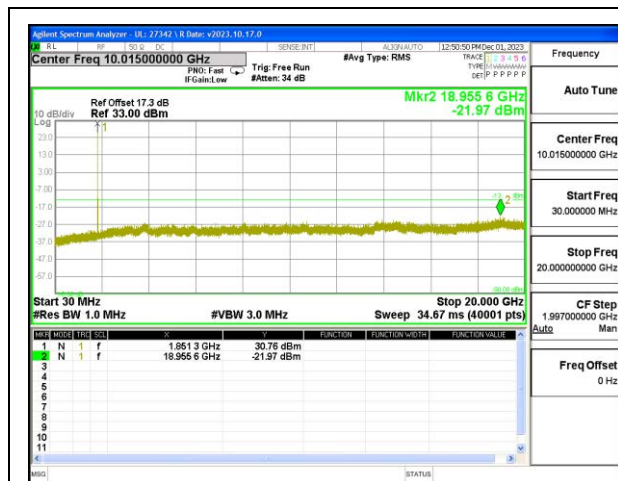
LTE B25 20MHz QPSK Low Channel RB1-0
