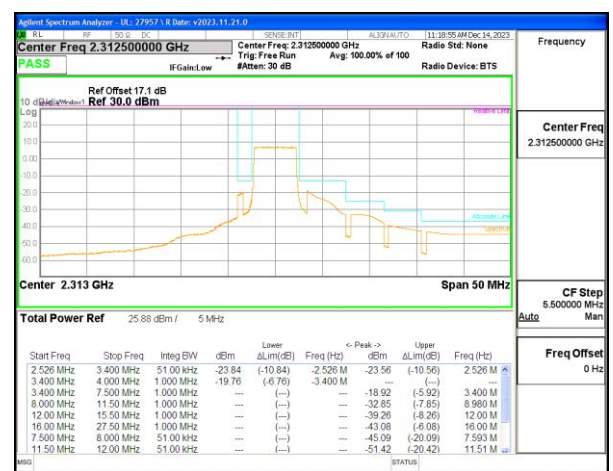
LTE B30 5MHz QPSK High Channel RB25-0 (High side)
