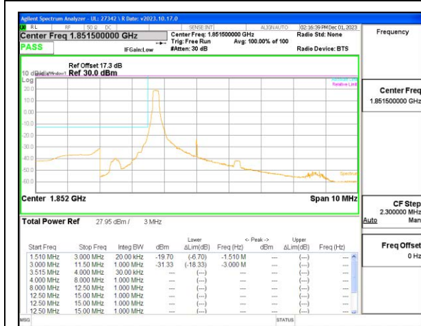
LTE B25 3MHz QPSK Low Channel RB1-0
