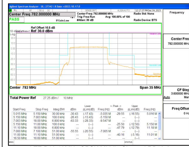
LTE B13 10MHz QPSK Middle Channel RB50-0
