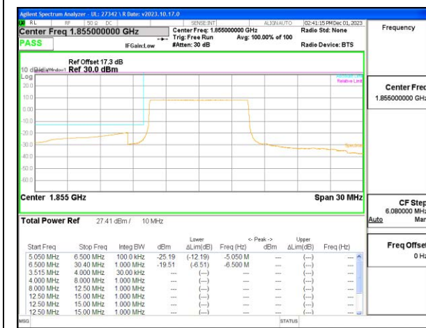
LTE B25 10MHz QPSK Low Channel RB50-0
