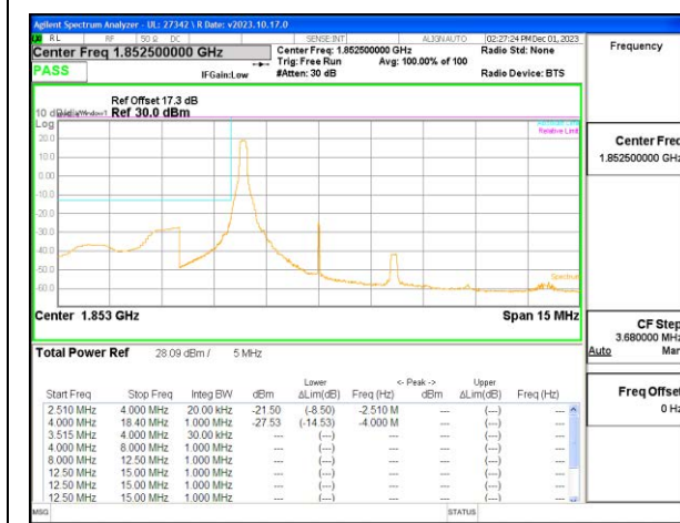
LTE B25 5MHz QPSK Low Channel RB1-0
