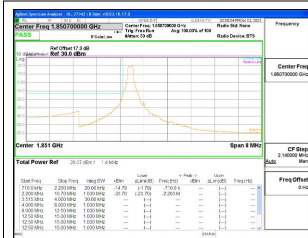
LTE B25 1.4MHz QPSK Low Channel RB1-0
