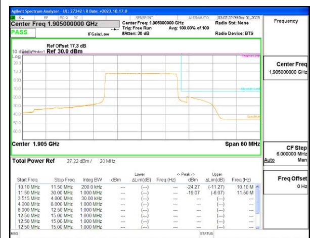
LTE B25 20MHz QPSK High Channel RB100-0
