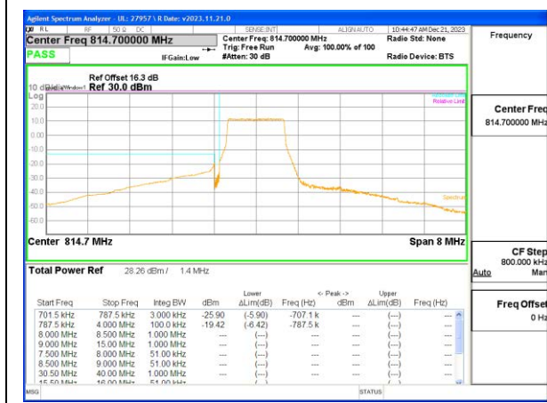
LTE B26 1.4MHz QPSK Low Channel RB6-0
