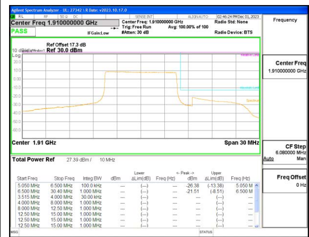
LTE B25 10MHz QPSK High Channel RB50-0
