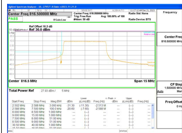
LTE B26 5MHz QPSK Low Channel RB25-0
