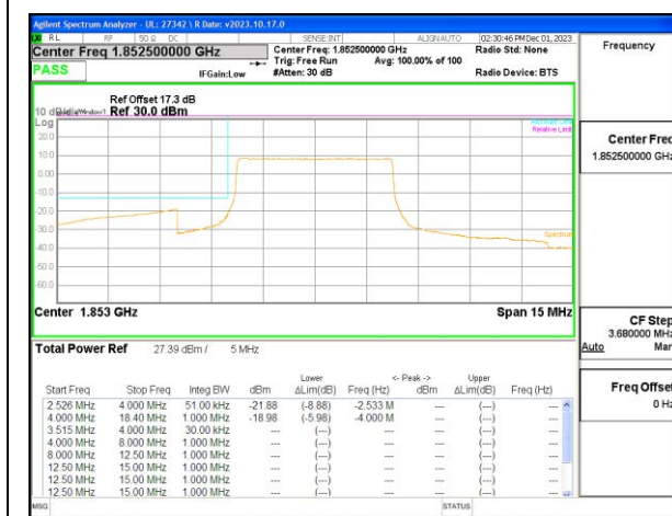
LTE B25 5MHz QPSK Low Channel RB25-0
