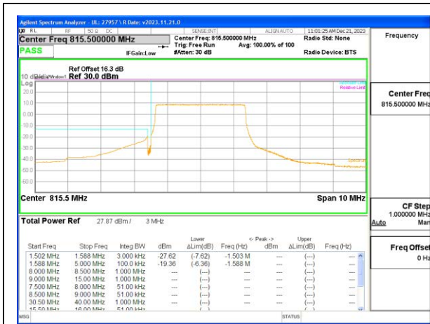
LTE B26 3MHz QPSK Low Channel RB15-0
