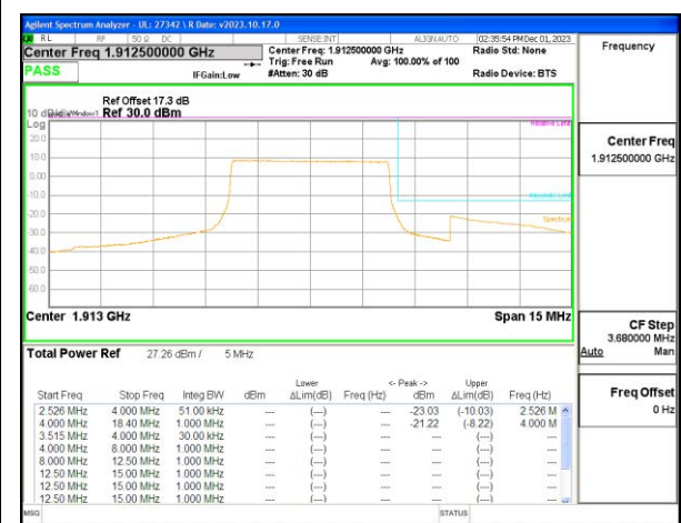
LTE B25 5MHz QPSK High Channel RB25-0
