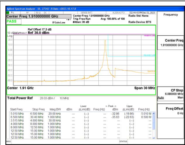
LTE B25 10MHz QPSK High Channel RB1-49
