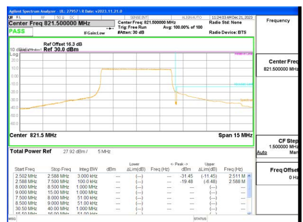
LTE B26 5MHz QPSK High Channel RB25-0
