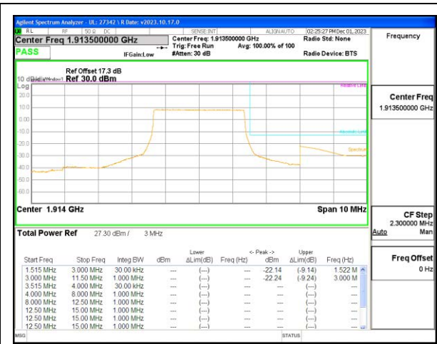
LTE B25 3MHz QPSK High Channel RB15-0
