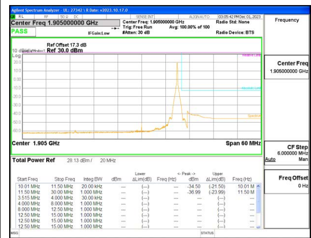
LTE B25 20MHz QPSK High Channel RB1-99
