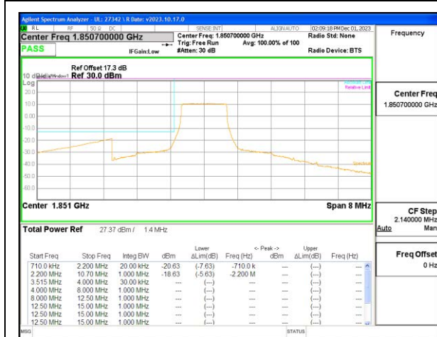
LTE B25 1.4MHz QPSK Low Channel RB6-0
