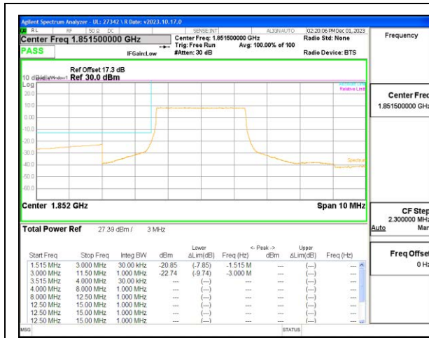
LTE B25 3MHz QPSK Low Channel RB15-0
