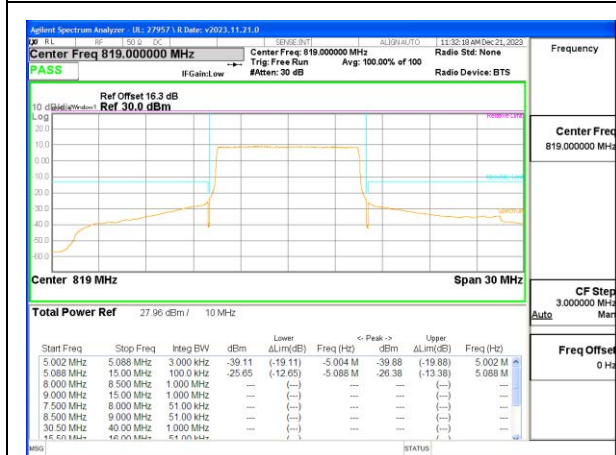
LTE B26 10MHz QPSK Middle Channel RB50-0
