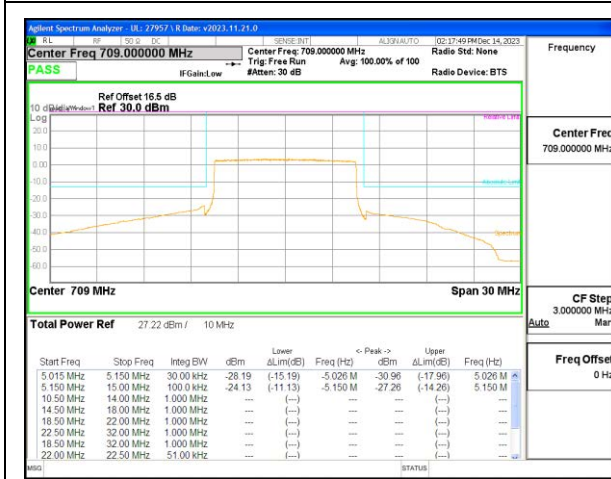
LTE B17 10MHz QPSK Low Channel RB50-0
