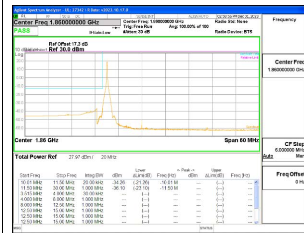
LTE B25 20MHz QPSK Low Channel RB1-0
