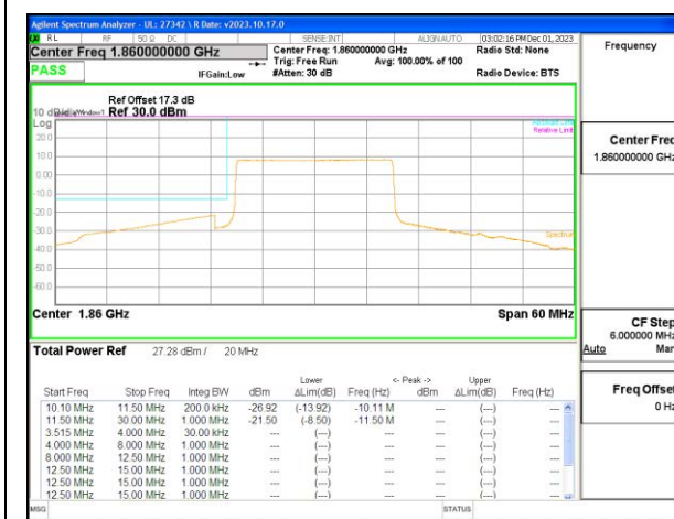
LTE B25 20MHz QPSK Low Channel RB100-0
