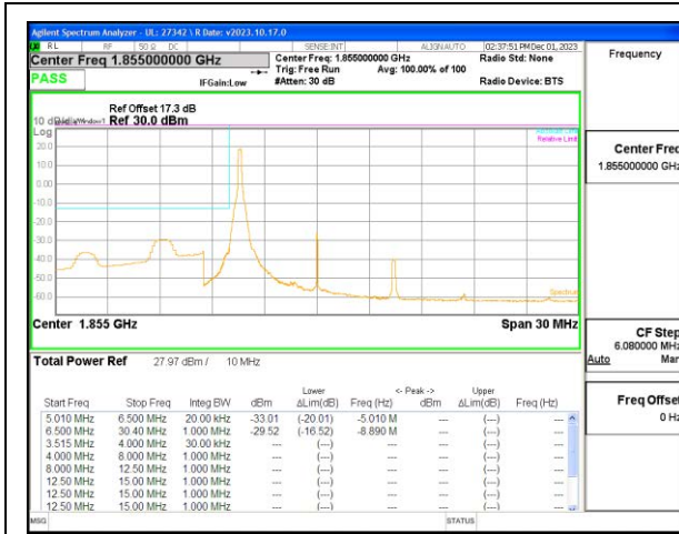
LTE B25 10MHz QPSK Low Channel RB1-0
