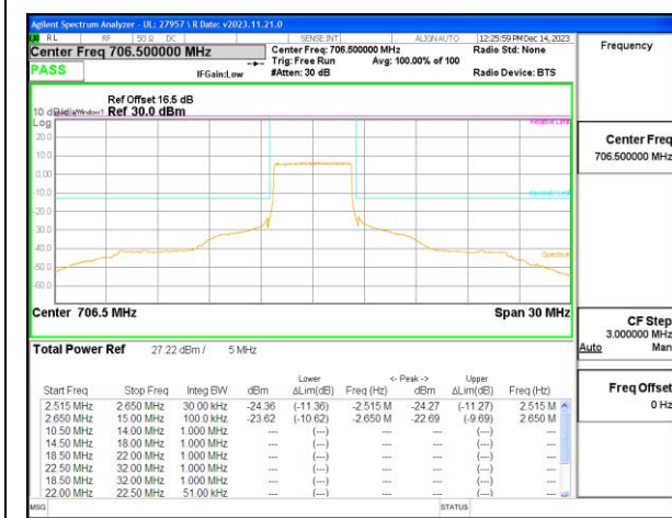
LTE B17 5MHz QPSK Low Channel RB25-0
