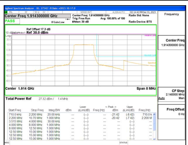
LTE B25 1.4MHz QPSK High Channel RB6-0
