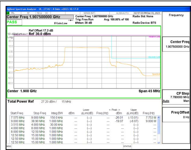
LTE B25 15MHz QPSK High Channel RB75-0
