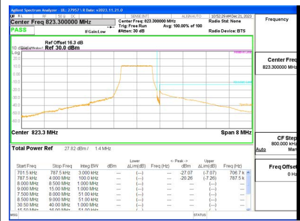
LTE B26 1.4MHz QPSK High Channel RB6-0
