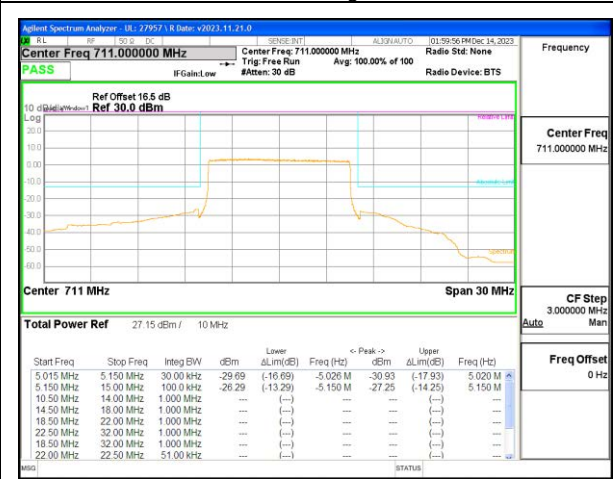
LTE B17 10MHz QPSK High Channel RB50-0
