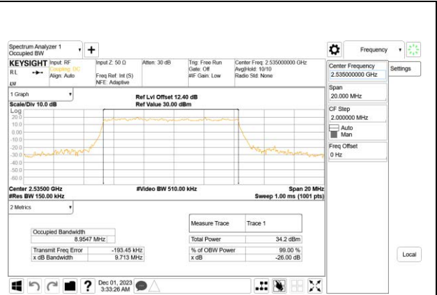
5G NR n7 10MHz BPSK Middle Channel RB50-0, ID: 27957
