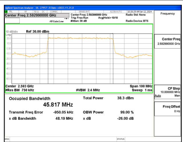
5G NR n41 50MHz BPSK Middle Channel RB128-0
