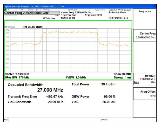
5G NR n41 30MHz BPSK Middle Channel RB75-0
