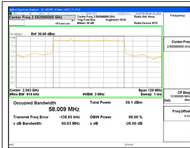
5G NR n41 60MHz BPSK Middle Channel RB162-0
