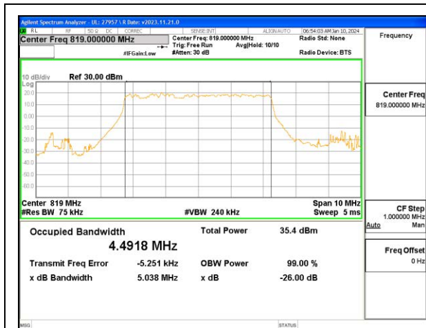
5G NR n26 5MHz BPSK Middle Channel RB25-0
