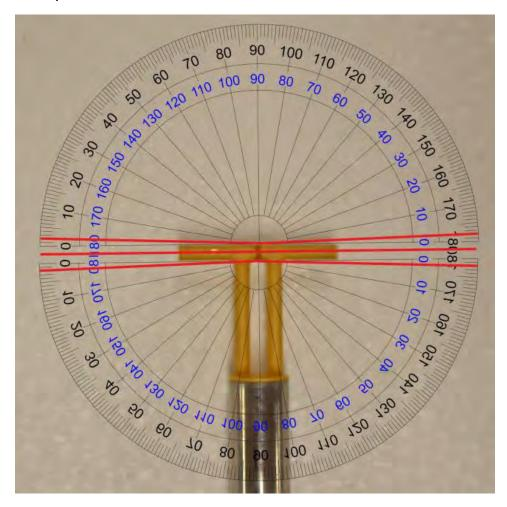
• The center red line indicates that the arms of the dipole fall within  $\pm 2^{\circ}$
