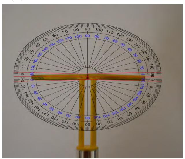
• The center red line indicates that the arms of the dipole fall within  $\pm 2^{\circ}$
