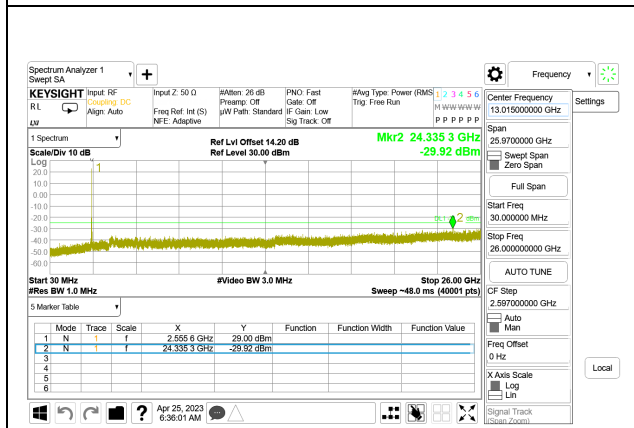
LTE B7 15MHz QPSK High Channel RB1-0, ID:19210
