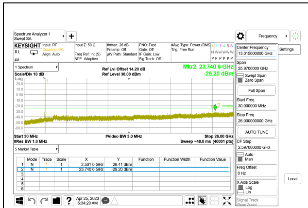
LTE B7 15MHz QPSK Low Channel RB1-0, ID:19210
