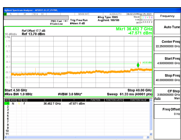
5G NR n48 30MHz BPSK Low Channel RB1-0 (4.5G to 40G)
