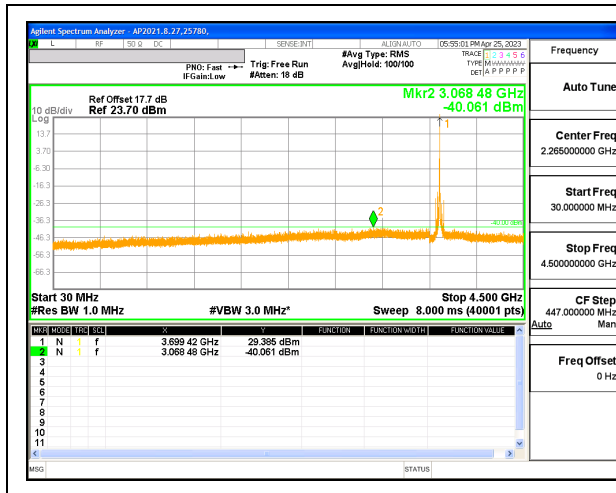
5G NR n48 40MHz BPSK High Channel RB1-105 (30MHz to 4GHz)
