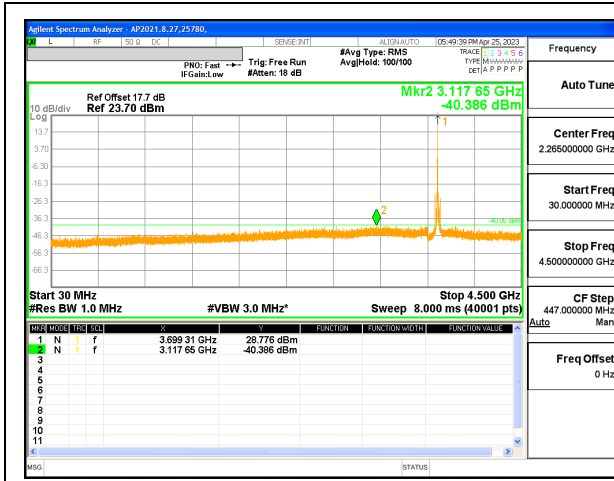
5G NR n48 30MHz BPSK High Channel RB1-77 (30MHz to 4.5GHz)
