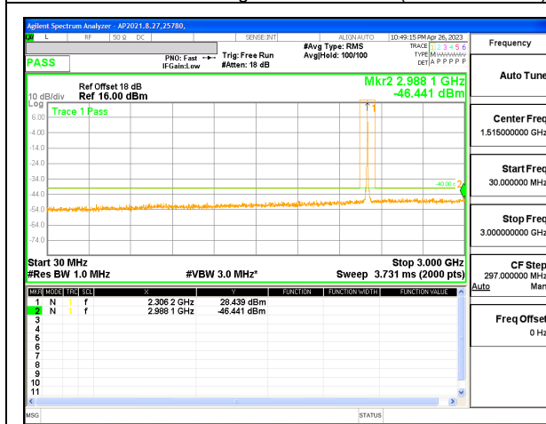
LTE B30 10MHz QPSK Mid Channel RB1-0 (30MHz to 3GHz)
