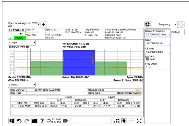
5G NR n48 40MHz BPSK Low Channel RB100-0
