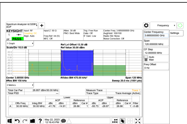
5G NR n48 30MHz BPSK High Channel RB1-0
