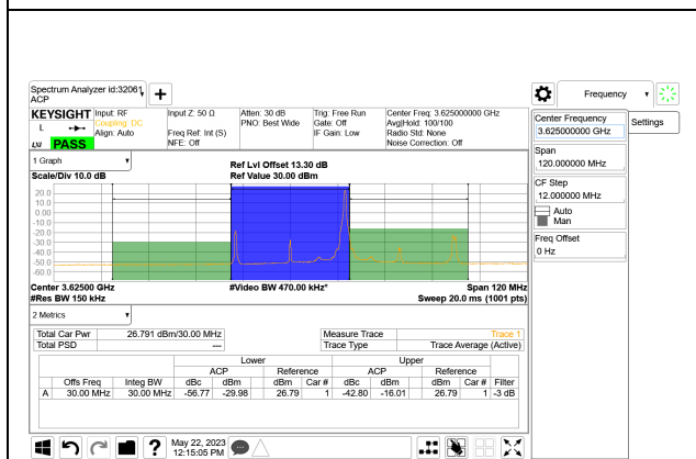
5G NR n48 30MHz BPSK Middle Channel RB1-77
