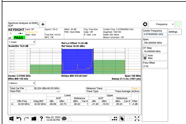
5G NR n48 40MHz BPSK Low Channel RB1-105
