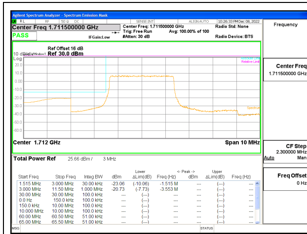
LTE B66 3MHz QPSK Low Channel RB15-0, ID:25780
