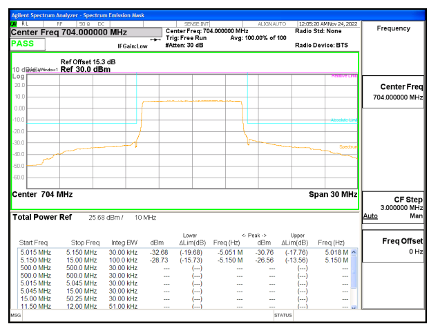
LTE B12 10MHz QPSK Low Channel RB50-0, ID:25780
