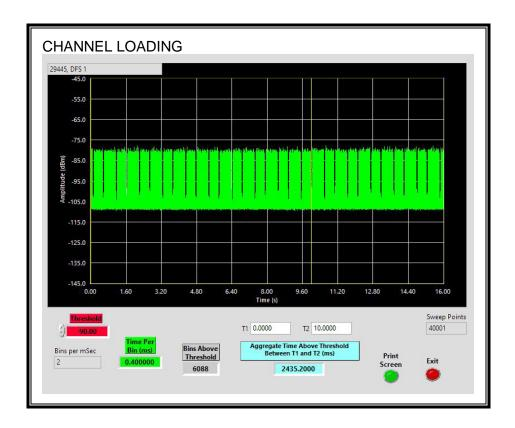
The level of traffic loading on the channel by the EUT is 24.35%
