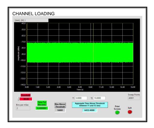
The level of traffic loading on the channel by the EUT is 64.32%
