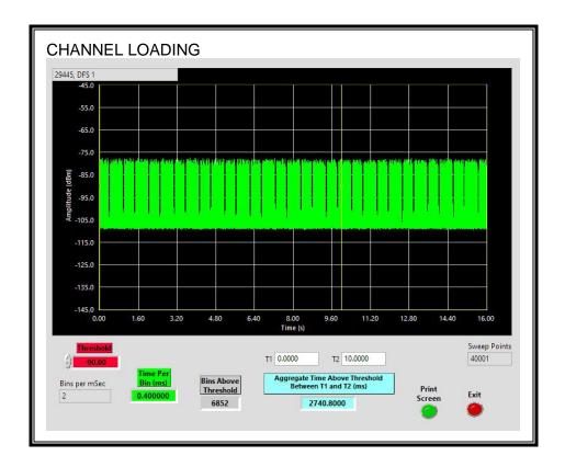
The level of traffic loading on the channel by the EUT is 27.4%
