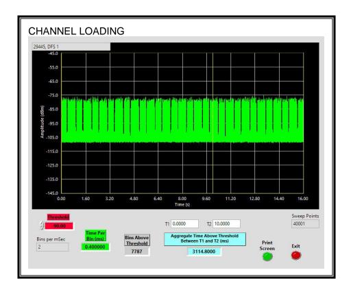
The level of traffic loading on the channel by the EUT is 31.14%
