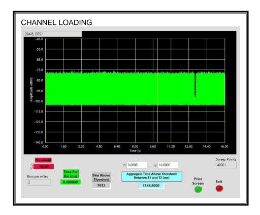
The level of traffic loading on the channel by the EUT is 31.88%
