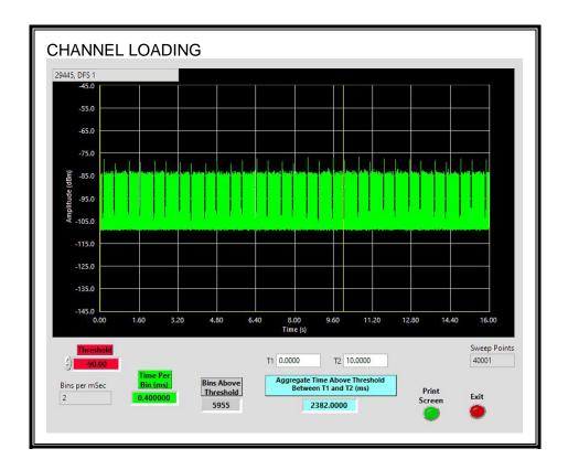
The level of traffic loading on the channel by the Peer Slave is 23.82%
