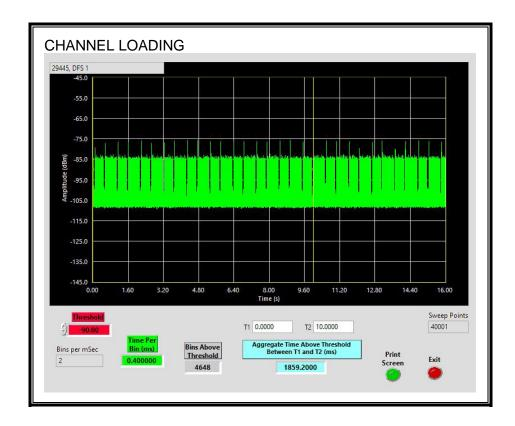
The level of traffic loading on the channel by the Peer Slave is 18.59%
