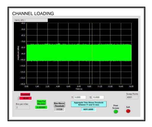
The level of traffic loading on the channel by the EUT is 46.91%
