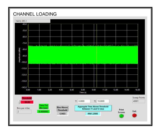
The level of traffic loading on the channel by the EUT is 49.61%
