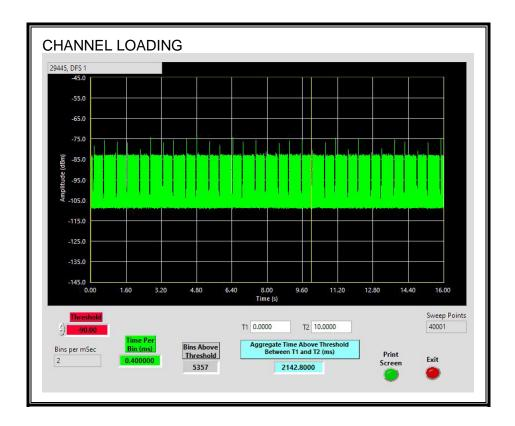
The level of traffic loading on the channel by the Peer Slave is 21.42%
