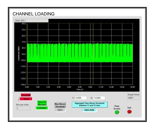
The level of traffic loading on the channel by the EUT is 28.84%
