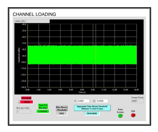
The level of traffic loading on the channel by the EUT is 28.18%
