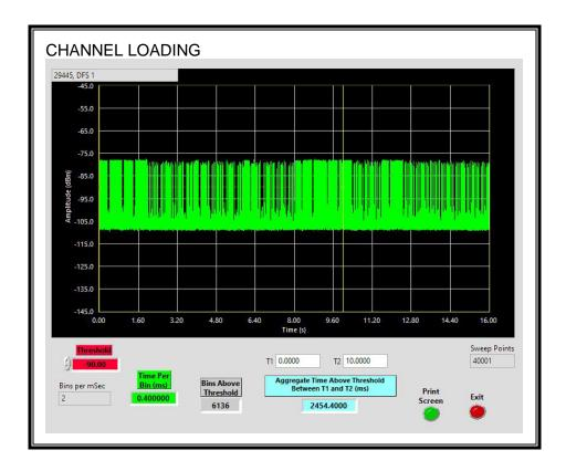
The level of traffic loading on the channel by the EUT is 24.54%
