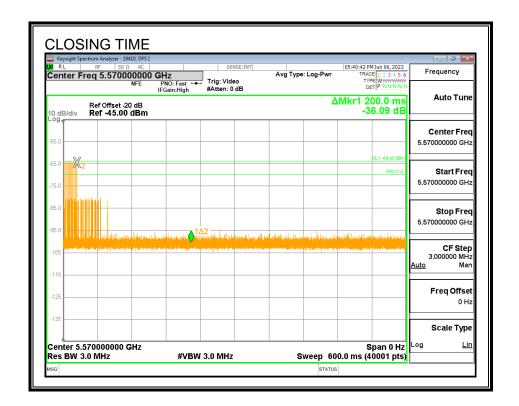
No transmissions are observed during the aggregate monitoring period.
