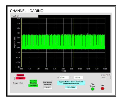
The level of traffic loading on the channel by the EUT is 24.99%
