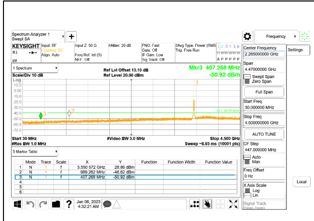
5G NR n48 10MHz BPSK Low Channel RB1-0 (30MHz to 4GHz), ID:28498
