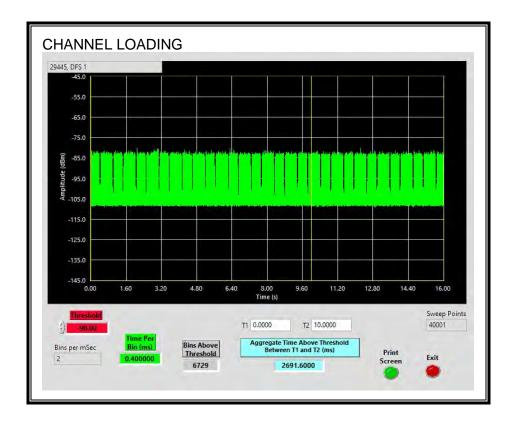
The level of traffic loading on the channel by the EUT is 26.91%
