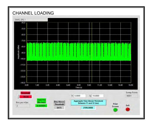
The level of traffic loading on the channel by the EUT is 25.9%
