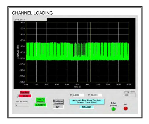
The level of traffic loading on the channel by the EUT is 32.17%
