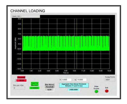
The level of traffic loading on the channel by the EUT is 24.88%
