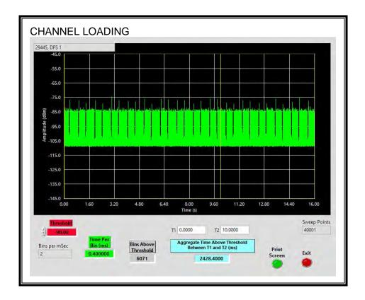
The level of traffic loading on the channel by the Peer Slave is 24.28%
