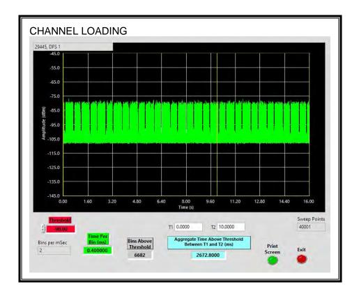
The level of traffic loading on the channel by the EUT is 26.72%
