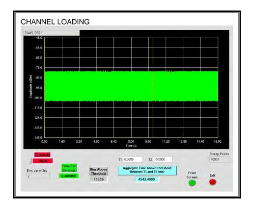
The level of traffic loading on the channel by the EUT is 45.42%
