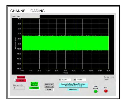
The level of traffic loading on the channel by the EUT is 24.96%
