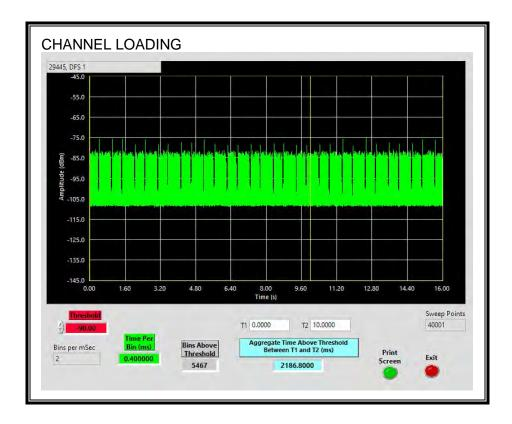
The level of traffic loading on the channel by the Peer Slave is 21.86%
