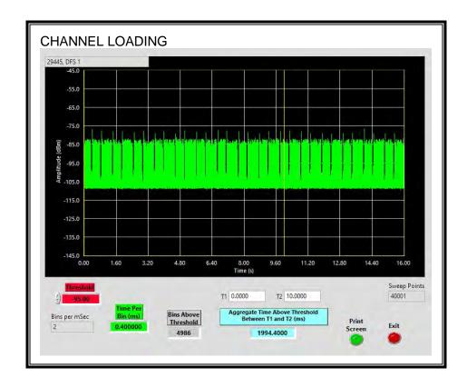
The level of traffic loading on the channel by the Peer Slave is 19.94%
