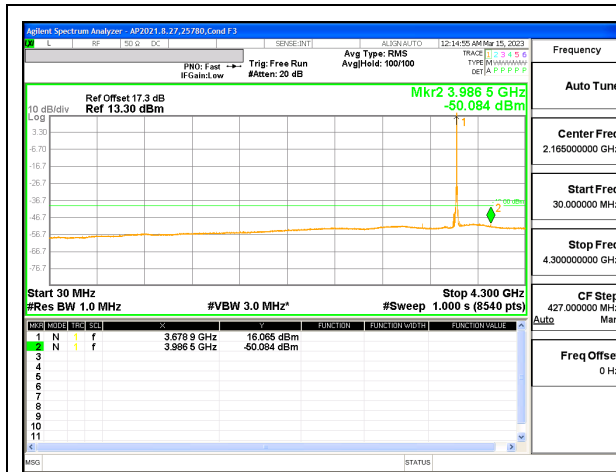
LTE B48 20MHz + 20MHz QPSK High Ch RB1-99 + RB1-0 (30MHz to 4.5GHz)
